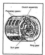
Direct drive power shift transmission was designed specifically for motor graders. It has no torque converter to cause lags or surges, just smooth no-clutch one-lever shifting with direct drive feel. Compact planetary gear sets provide high reduction in minimum space. large diameter clutch assemblies have high holding capacity. Plates are continuously lubricated and cooled by oil.
