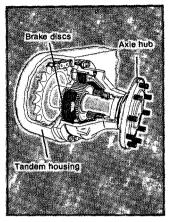
Four-wheel oil disc brakes are bathed in oil and sealed to the environment. They need none of the periodic adjustment and lining replacement typical of shoetype brakes. Each tandem set is activated by its own air circuit, so failure in one circuit still leaves half the original braking capacity. ROPS cab or canopy, work lights, directional signals, other safety items are all available for specific user needs.
