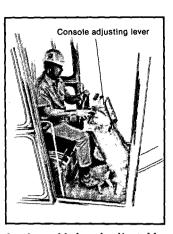
deeply padded and adjustable. Blade levers are arranged in the familiar Caterpillar pattern for easy operator orientation. Transmission control is a single lever to the operator's right. It's full power shift — no manual clutching — so he can shift up or down without stopping the machine or losing time or momentum. An "inching" pedal lets him ease up to curbs or obstructions.
